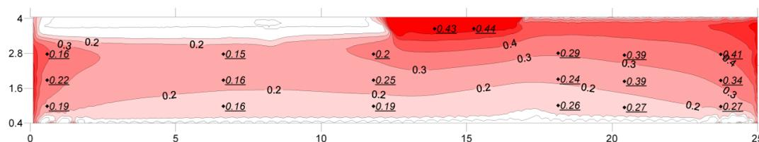
Figure 1. Results from two-phase simulations on the test facility. The contour map shows simulation results while the underlined values show the measured results.
