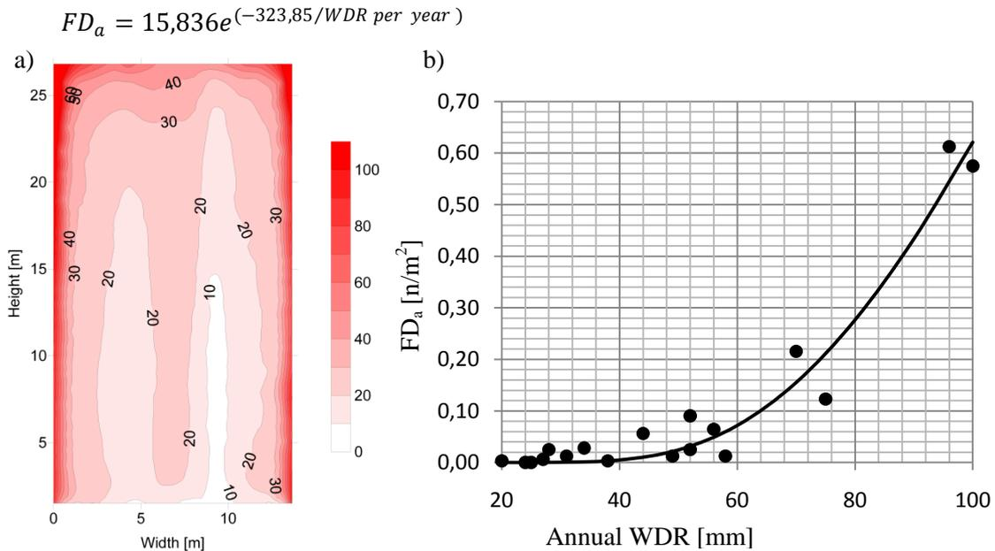
Figure 2. Figure a) shows the total average annual amount of WDR impinging on the north facade. Figure b) shows the annual amount of WDR plotted against the annual amount of frost damage on the wall.
